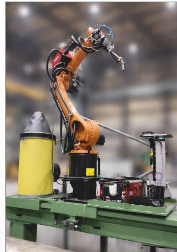
Drupe Tracks Not only extend working area but also expands endless possibilities like accelerations speeds upto 3m/s<sup>2</sup> repeatability upto  $\pm 0.02$ mm and industrial leading performance. Our Tracks supports range of robots. Using single robot and Drupe Tracks it greatly utilizes automation process.
